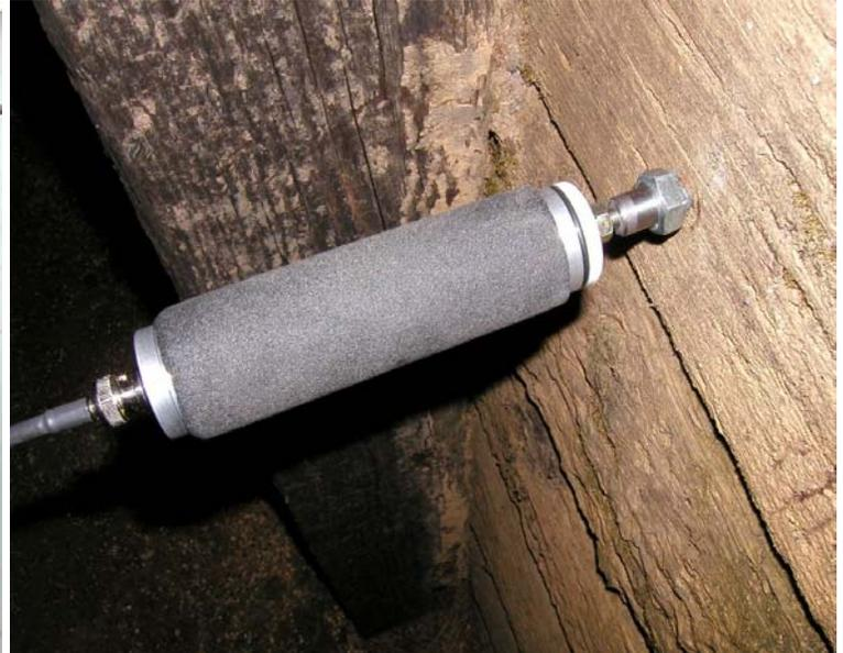
Model SP-1 probe modified for use with a high intensity rare earth magnet to attach to a lag bolt screwed into wooden beam. This probe design can also be used on trees and for soil applications where lag bolts can be conveniently inserted to different depths. The magnet is  $\frac{1}{2}$ " diam and has a pull of 15 lbs.
