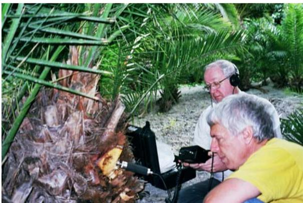
Dr. Roger Hill (back) and Dr. Michel Ferry listen to one of the palm trees. The SP-1 sensor is magnetically attached to a nail that has been inserted into the soft palm wood. The nail acts as a “waveguide” to conduct the sounds to the SP-1 sensor from RPW larvae feeding on the wood.
