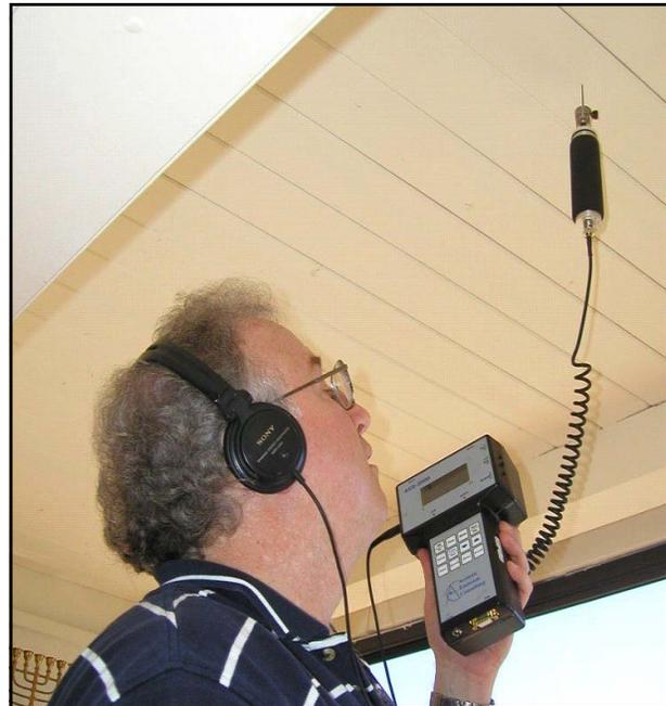
Listening to drywood termites in a porch tongue-and groove ceiling. A 1/16" drill bit inserted into the wood is attached with the drill bit adaptor and magnet to the SP-1L probe. This method is also used through drywall.
