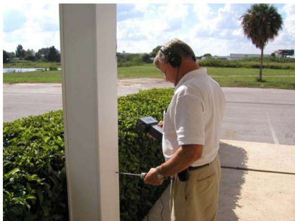
Probing for drywood termite activity on a wood column with rubber-tipped SP-1L probe.
